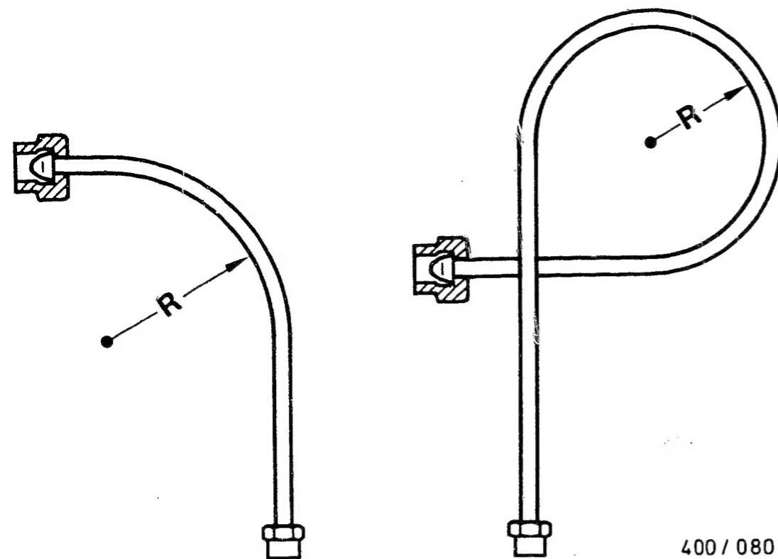
Min. perm. bending radii for calibrating fuel-injection tubing:
